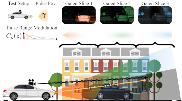
Figure 2. Gated Image Formation and Bi-Directional Sampling. Top-row: Our test vehicle is equipped with a synchronized stereo camera setup and illuminator that flood-lits the scene with a light pulse and FoV \gamma . Using different gating profiles C(z) , we capture three slices with intensity visualised here in red, green and blue. Illustrated in the middle row, the gating profiles describe pixel intensity for a point at sensor distance z . The first slice (red) accounts for close ranges, the green for mid-ranges, and the blue for far ranges. Bottom-row: we show the ray sampling employed in our method, based on a bidirectional sampling strategy. We cast the rays from the illuminator view to explore the occluded areas, while the rays casted from the camera integrate the reflected scene response. The shadowed areas are marked in gray.
