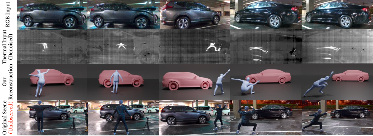
Figure 6. Real-world 3D human reconstruction from thermal reflections of cars. A diverse set of human poses can be reconstructed by using the surfaces of different types of cars as infrared mirrors. RGB input (1st row) and thermal input (2nd row) captured by a depth camera and a thermal camera are used as input to our method. Our reconstruction (3rd row) is compared with the original scene (4th row), both rendered/captured from another camera viewpoint.
